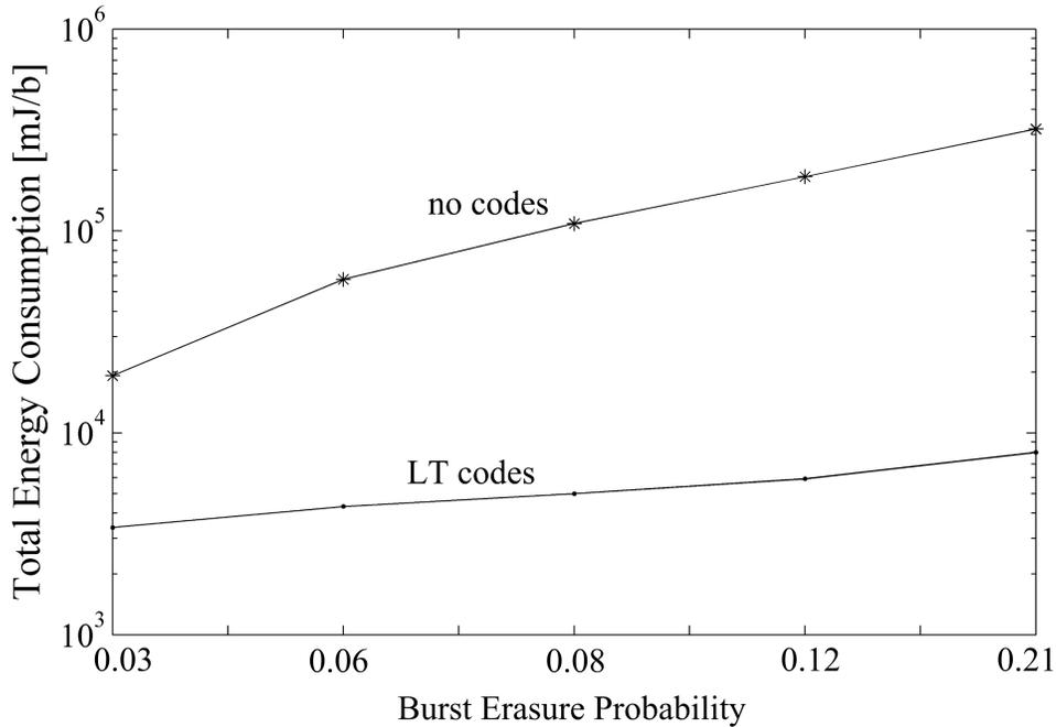
Fig. 5. Energy consumption of LT codes compared to energy consumption of transmission without coding schemes. The basic retransmission policy considered, retransmits all the source block if packets are lost.
