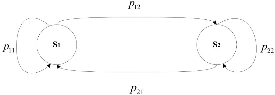
Fig. 3. Markov binary process, which models the burst packet erasure channel. The system can be either in the states  $S_1$  or  $S_2$ , which are respectively the error-free state and the one in which packets are erased. Next, conditional probabilities  $p_{12}$  and  $p_{21}$  are the transition probabilities and  $p_{11}$ ,  $p_{22}$  are the probabilities of keeping the system in the current state.
