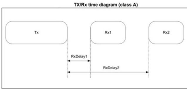
**Figure 3.** LoRaWAN Class A Devices.
