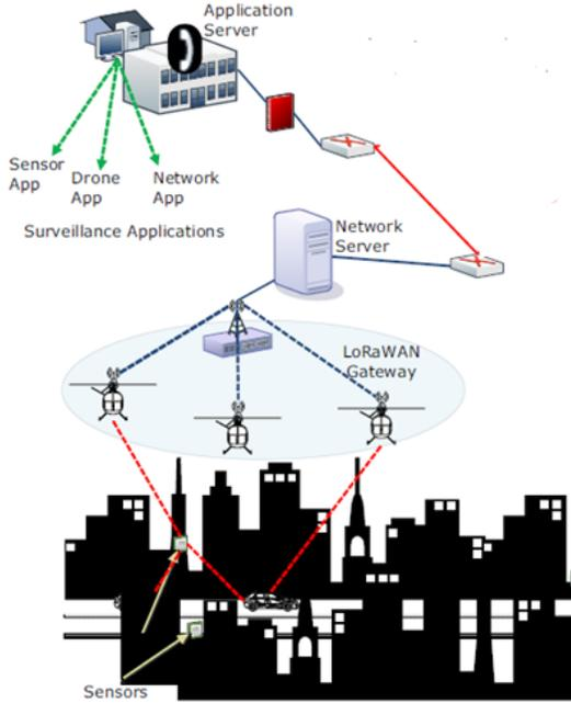
Figure 12. Scenario with LoraWAN Gateway mounted on a drone.
