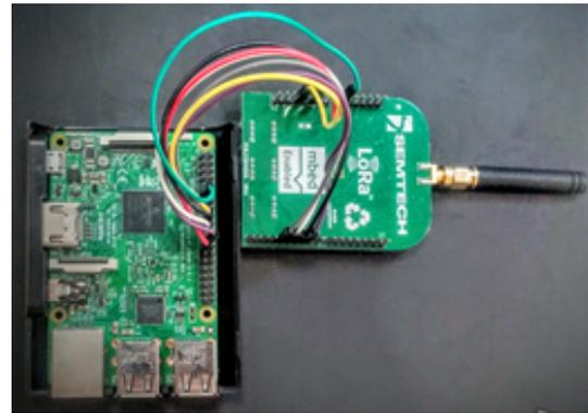
**Figure 5.** Hardware components of LoRa gateway.
