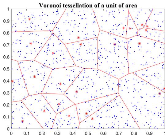
**Figure 14.** Voronoi tessellation, which provides a snapshot of the coverage of a unit of area. The red stars are the mobile BSs while the blue dots are the peripherals.
