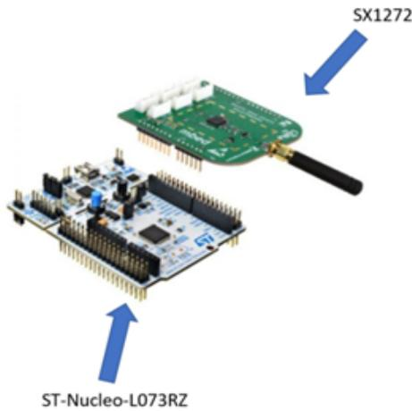
**Figure 4.** Hardware components of LoRa sensor communication section.
