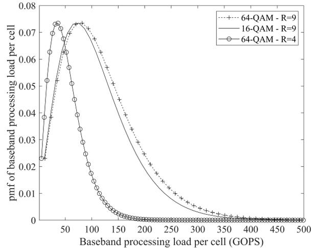
Fig. 3. Probability mass function of baseband processing load per cell.
