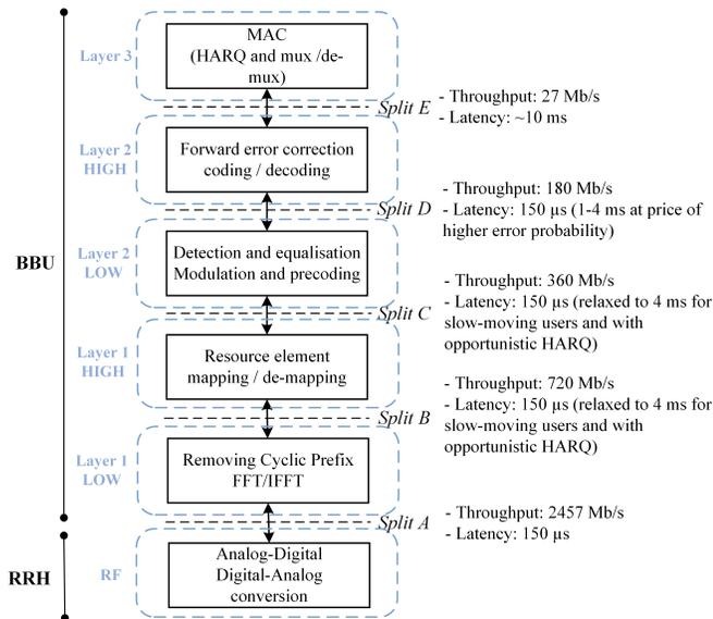
Fig. 1. Functional architecture of radio and baseband unit (uplink and downlink), considering the possible split points. On the right side, the backhaul requirements for C-RAN split options [4], [5].
