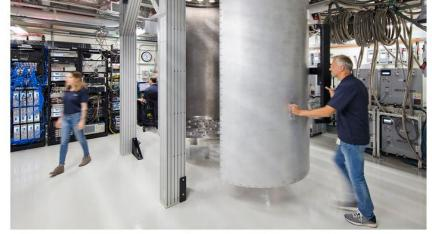
IBM researchers have already installed the mounting hardware for a jumbo cryostat big enough to hold a guantum computer with 1 million gubits. CONNIE ZHOU/IBM
